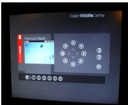
The camera is controlled by visitors using a touchscreen LCD display with a built in video window. One of the advantages with the touchscreen is that it can be customised and remotely updated to accommodate extra cameras in the future. There is also a camera control console fitted with a joystick for staff use, this allows more in depth control of camera settings.
